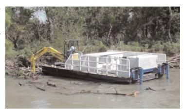
The unique design of the steering and propulsion system allows the barge to easily navigate within the narrow stretches of the river channels.
